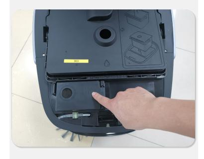
2.Press the clips inward, and open the air filter cover;
