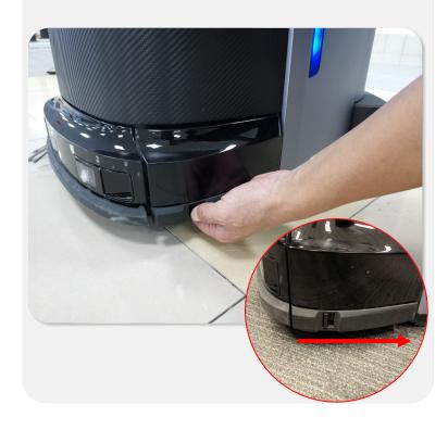
**2.**Press the button and take the dust collector out.
