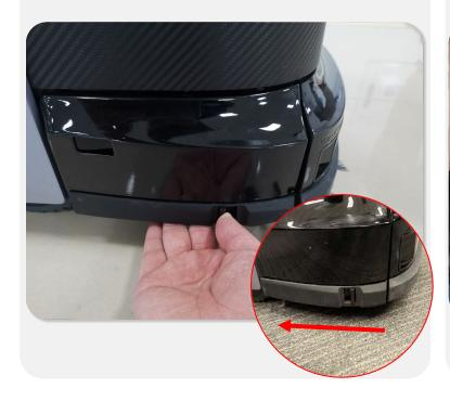
2.Grab the rubber boot and pull down to remove the side brush.
