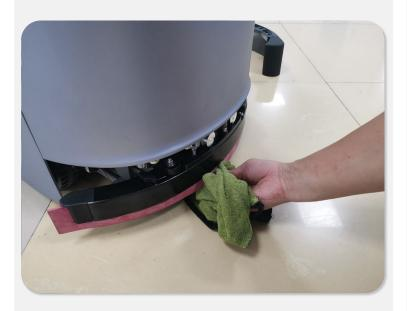
**2.**Clean the gap between the inner and outer strips.
